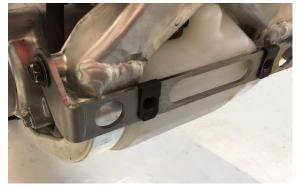
Note-If weld slag impairs fit of the bracket, dress down the slag area with a flat file just enough to allow proper fit.
